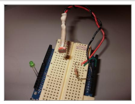
Use the breadboard (or protoshield) to connect one leg of the photoresistor to Analog Input 0, and the other leg to +5v. Then, take the 10K resistor and connect one leg to GND (ground) and the other to Analog Input 0. Also, I wired an LED to Digital I/O pin 13 to show when the laser beam is broken. Hook the negative end of the LED to ground as well.
